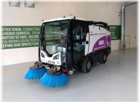
invaluable tool to keep the carparks clean. Not only does in it have front brushes and a large vacuum unit for cleaning large areas, it also comes equipped with a wonder hose and lance, which can be used to remove litter from tight spots and wash down difficult to reach areas such as stair wells.
